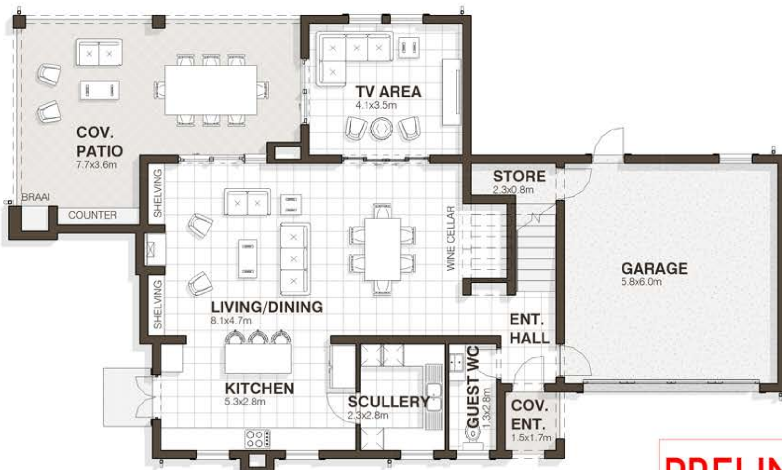
GROUND STOREY PLAN SCALE 1 : 100
